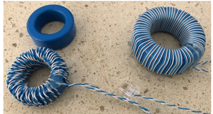
Figure 2 Example DIY common mode chokes and a bare N30 ferrite toroid
