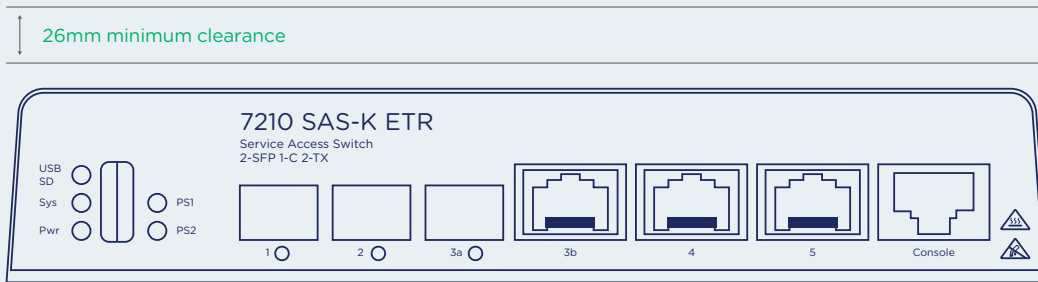
Figure 2b. BNTD cooling fins clearance requirements
