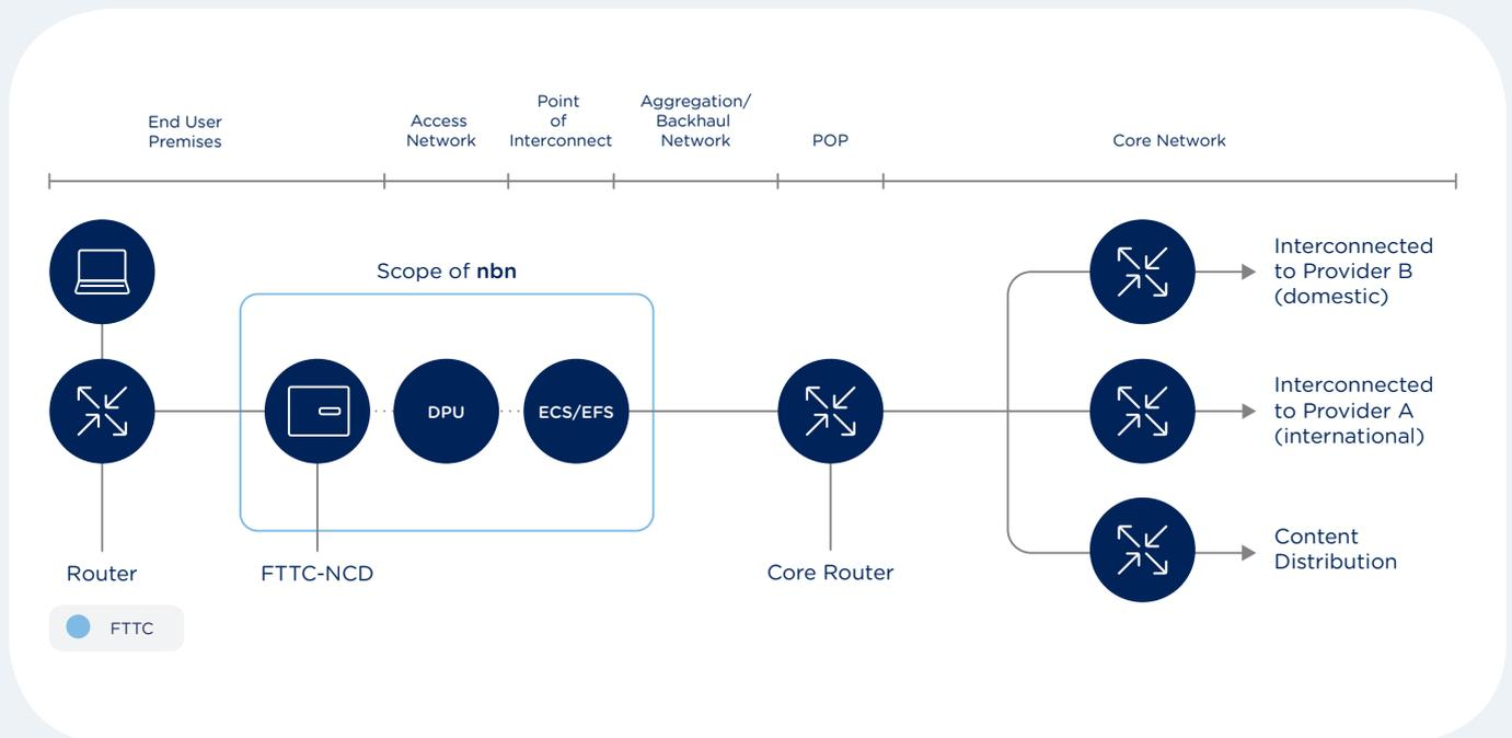
For the Service Provider, the use of an **nbn**<sup>TM</sup> Ethernet (FTTC) will see the modification, replacement or elimination of certain copper access components:
